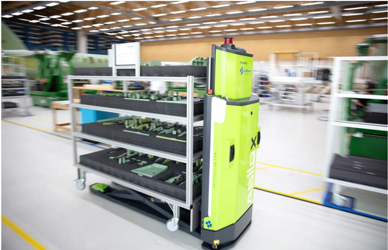
Driverless transport system in the structural assembly hall
